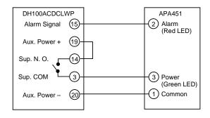
NOTE: Wiring diagram shown is for DH100ACDCLWP 4-wire duct smoke detector system equipped without a control panel.
